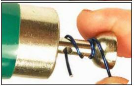
5. Wrap the wire around the mandrel with your dominant hand while holding the tool with your non-dominant hand. Or turn the tool with your dominant hand and guide the wire onto the mandrel with your non-dominant hand. Switch these positions to find the method that you prefer.
