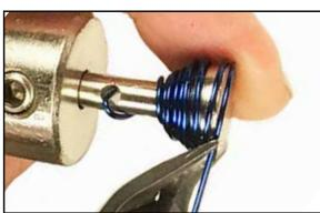
7. Trim the end of the wire with a Flush Cutter, then cut the wire at the hole of the mandrel.
