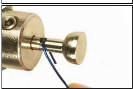
3. Place the end of a piece of wire (approximately 12 inches long) into the guide hole in the mandrel shank and bend the wire, as shown.
