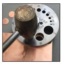
**Step 4** – Cut as many discs as you will need to go with your chosen accent beads. I made 6 pairs for this tutorial so I cut 12 discs before moving on.
