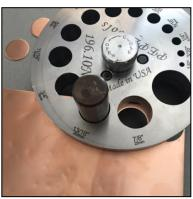
**Step 3** – Use a heavy brass hammer to hit the punch once or twice to cut out your disc.
