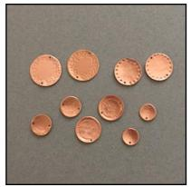
**Step 8** – Dap your discs. Using a wooden dapping kit and a rubber or rawhide mallet, hammer until the disc is evenly domed. Start working in a depression that seems large and move progressively to smaller ones to get the best shape.
