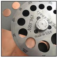
**Step 2** – Insert the punch that corresponds to the hole size. The right punch will fit perfectly with no wiggle room.
