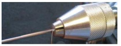
to hold it. Spin the handle to coil the wire around the length of the base wire. Repeat for the number of wires you want to use. For this project, I used 14.
