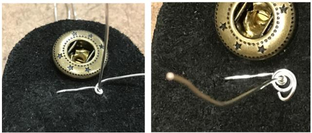
13.Bend the second wire over and under the first to create a coil around the first.
