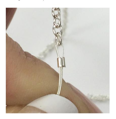
6. Follow your crimper's directions to crimp the tube or bead. I'm using the Om Tara Crimpers that work on any size crimp. First I crimp the beading wire, making sure the wires don't cross over each other.
