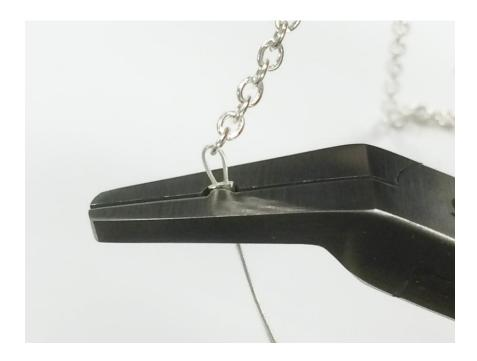
7. Next turn the crimped wire to the side and press the crimp closed. Don't squeeze overly hard.
