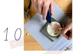
Using wire rounder/dremel in shallow dish of water, round off the end of the wire so it's ready to wear!
