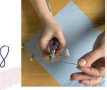
Curve wire over until back of wire is parallel with front.
