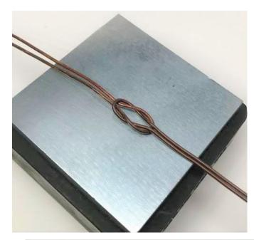
4. Link the two wire sections together to form a square knot or "reef knot" by placing the tails of one piece down through the loop of the other piece and the tails of that piece up through the loop of the other piece.
