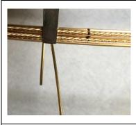
Find the middle of your stack. Hook your binding wire over that middle and hold with your flat pliers. Come from the bottom or the top. Find which is more comfortable for you.
