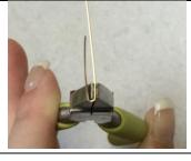
Use the end of your flat nose pliers to bend a U shape into your binding wire. Make sure the flat side is on the inside.
